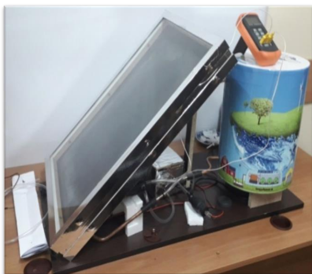
Fig. 6. Type 3 – Solar collector mockup with chemical coating
